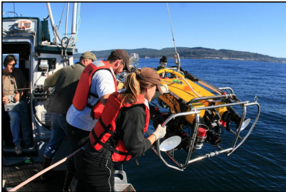
This remotely operated vehicle (ROV) is a tool ODFW uses to survey the ocean bottom and its inhabitants. Photo Credit: ODFW.
