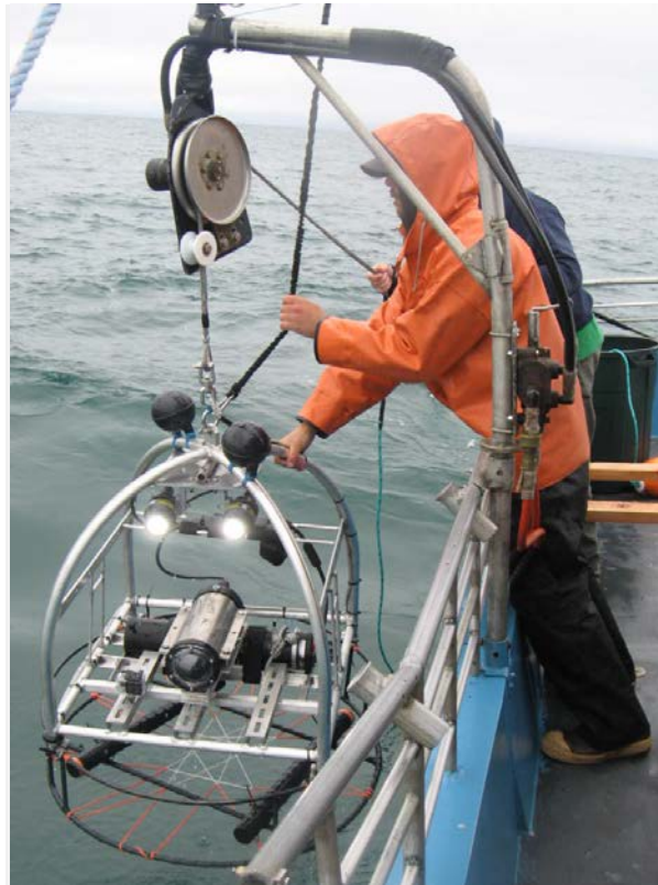
A video lander designed by ODFW being retrieved after sampling rocky subtidal habitat. Photo Credit: ODFW
